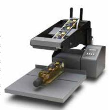
Operation is simple: place the container in the mechanism and pull the arm to the container and the label is automatically applied. Variable spacing, memory for up to nine different containers, and a counter with built-in LED display are all included. No air-pressure supply is required which can be a significant advantage over other label applicators that require expensive, noisy and maintenance -prone air compressors.
